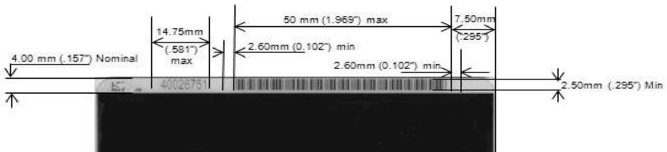
Figure 1 – Barcode and Serial Number Placement and Dimensions
